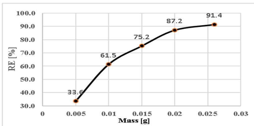
**Figure 3.** The removal efficiency (RE) of BB during 2h at pH 9 on various amount of Fe<sub>3</sub>O<sub>4</sub> nanomaterial (0.005, 0.01, 0.01, 0.02 and 0.025 g)
