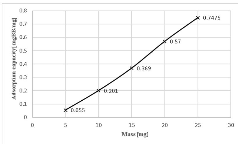
**Figure 4.** BB1 adsorption capacity by 5-10-15-20-25 mg magnetite nanomaterial (Fe<sub>3</sub>O<sub>4</sub>) during 2 h at pH 9
