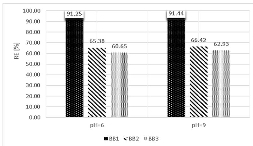
**Figure 2.** The influence of pH upon the removal efficiency (RE) % of BB by the nanomaterial
