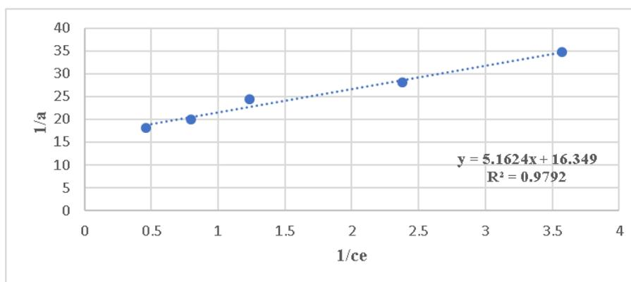
**Figure 5.** Variation of the Langmuir adsorption isotherm of benzalkonium bromide on magnetite nanomaterial
